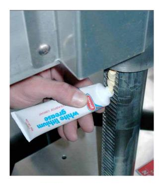
LUBRICATE SHAFT AND TEETH WITH WHITE LITHIUM GREASE EVERY 6 MONTHS
