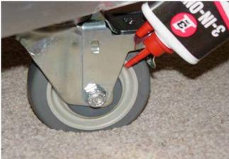
LUBRICATE TURNING POINT AND 4 WHEELS WITH 3 IN 1 OIL EVERY 6 MONTHS
